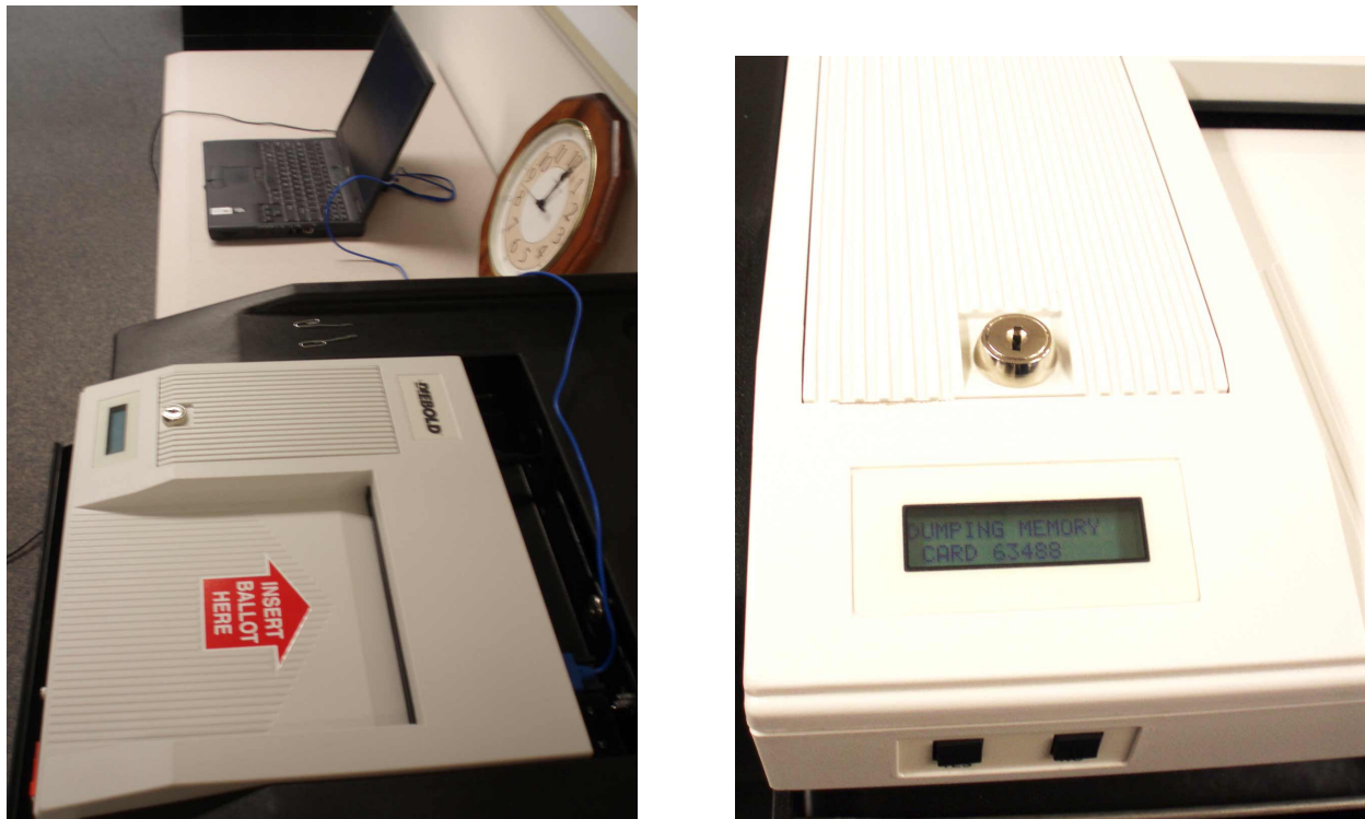
Figure 5: ( Left ): The setup for compromising the AV-OS. A standard laptop is connected through its serial port to the serial port of the AV-OS machine. ( Right ): Dumping the memory contents through the serial line. Anyone with physical access to the AV-OS can perform this operation since this function does not require any authentication. The number shown in the LCD screen is the amount of remaining bytes before the dump is completed (each card holds 128Kb of data).
