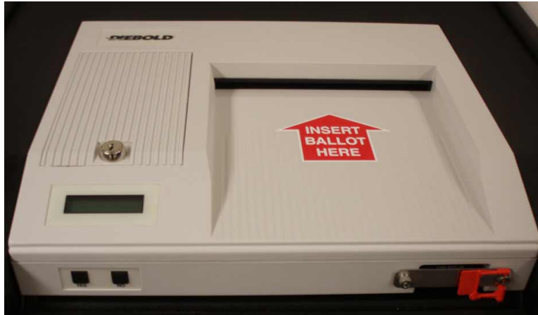
Figure 1: The AccuVote Optical Scan voting terminal (AV-OS). The terminal is shown prior to it being locked to the ballot box, with its front panel visible and showing two control buttons (lower left corner) and the memory card slot with the card sealed in (lower right corner).
