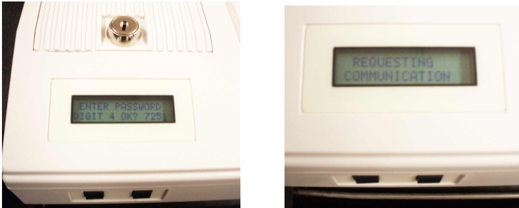
Figure 7: ( Left ) : The attacker enters the PIN to enter supervisor mode. ( Right ) : The AV-OS is requesting communication from the GEMS system to overwrite the memory card contents with the forged election setup.
