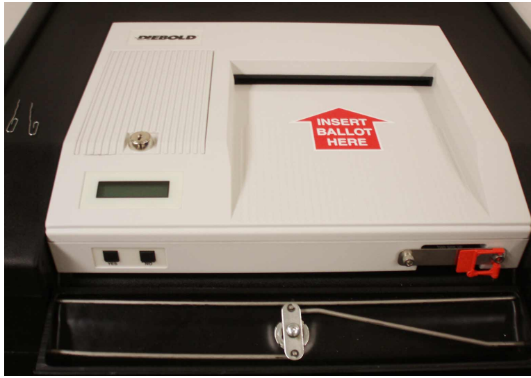
Figure 4: The front side of the AV-OS with the Yes/No buttons accessible.
