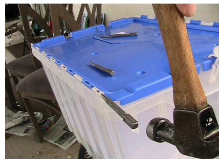
Drive the steel hinge pin out from the end opposite the "retaining curve". The plastic is easily flexible enough to bend around the steel "bump" without leaving a mark.
