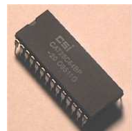
A standard EEPROM chip - something like this is inside the Sequoia memory pack...
